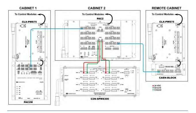
**NOTE:** If more than 50 watts of power is drawn by connected devices, supplemental power supplies are required.
